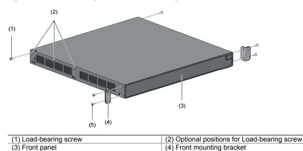
Figure 3-6 Fix front mounting brackets and load-bearing screws
